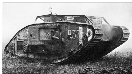
A British Mark V tank put out of action by the direct fire of a German “77” in the First World War. Although the tanks of this war had a mechanical endurance of about eight hours, the crews had incapacitating motion sickness after about two.
